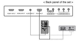
Connect the signal cable from the monitor output socket of the PERSONAL COMPUTER to the **RGB INPUT** socket of the set.
